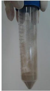
Figure 7 – Extracted and purified Kraft Lignin.
